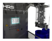
The HRS AF-1000 Series range of single and dual head aseptic fillers are designed for use with 'bag-in-box' and 'bag-in-drum' type aseptic packaging solutions. In the process, thermal sterilisation of the product is carried out separately from that of the package. Sterile conditions during the packaging process are maintained using steam, so that chilled or ambient temperature product can be put into the container without any contamination before the pack is sealed.
