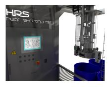
The HRS AF-1000 Series range of single and dual head aseptic fillers are designed for use with 'bag-in-box' and 'bag-in-drum' type aseptic packaging solutions. In the process, thermal sterilisation of the product is carried out separately from that of the package. Sterile conditions during the packaging process are maintained using steam, so that chilled or ambient temperature product can be put into the container without any contamination before the pack is sealed.
