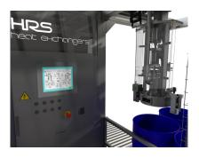
The HRS AF-200 Series range of single and dual head aseptic fillers are designed for use with 'bag-in-box' and 'bag-in-drum' type aseptic packaging solutions. In the process, thermal sterilisation of the product is carried out separately from that of the package. Sterile conditions during the packaging process are maintained using steam, so that chilled or ambient temperature product can be put into the container without any contamination before the pack is sealed.
