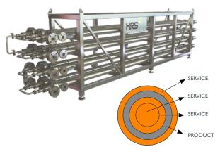
The HRS AS 4 Series is a complete stainless steel quadruple tube heat exchanger designed for applications with viscous fluids. The product flows through the annular spaces and the service fluid flows through the service tubes to ensure even heating or cooling. The removable inner tube allows for easy inspection of annular space. Using HRS' corrugation technology, heat transfer and efficiency are increased over standard smooth tube heat exchangers. In addition, effects of fouling are minimized.
