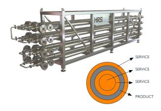
The HRS AS 4 Series is a complete stainless steel quadruple tube heat exchanger designed for applications with viscous fluids. The product flows through the annular spaces and the service fluid flows through the service tubes to ensure even heating or cooling. The removable inner tube allows for easy inspection of annular space. Using HRS' corrugation technology, heat transfer and efficiency are increased over standard smooth tube heat exchangers. In addition, effects of fouling are minimised.
