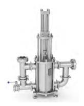
The HRS BP Series piston pump is a fully hygienic, hydraulically operated positive displacement pump. The pump is driven by a hydraulic power pack which drives a hydraulic cylinder from alternate directions, moving the piston up and down.
