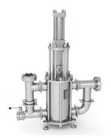
The HRS BP Series piston pump is a fully hygienic, hydraulically operated positive displacement pump. The pump is driven by a hydraulic power pack which drives a hydraulic cylinder from alternate directions, moving the piston up and down.
