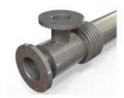
The HRS DTI Series is a complete stainless steel double tube heat exchanger designed for industrial and environmental applications. The product flows through the inner tubes and the service fluid flows through the surrounding shell. As a result of its geometry, the DTI Series has a continuous free-pass cross section allowing large particles to be processed and reduces the risk of product blockages.
