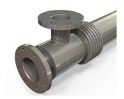
The HRS DTI Series is a complete stainless steel double tube heat exchanger designed for industrial and environmental applications. The product flows through the inner tube and the service fluid flows through the surrounding shell. As a result of its geometry, the DTI Series has a continuous free-pass cross section allowing large particles to be processed and reduces the risk of product blockages.
