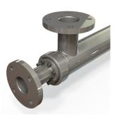
The HRS DTIR Series is a complete stainless steel double tube heat exchanger designed for industrial and environmental applications. The product flows through the inner tubes and the service fluid flows through the surrounding shell. As a result of its geometry, the DTIR Series has a continuous freepass cross section allowing large particles to be processed and reduces the risk of product blockages.
