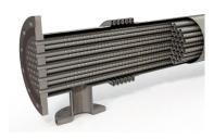
The HRS KHP Series is a complete stainless steel shell and tube heat exchanger designed for industrial use. The product flows through the inner tubes and the service fluid flows through the surrounding shell.
