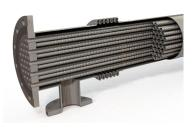
The HRS KHP Series is a complete stainless steel shell and tube heat exchanger designed for industrial use. The product flows through the inner tubes and the service fluid flows through the surrounding shell.
