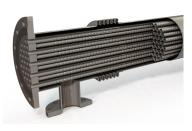
The HRS K Series is a complete stainless steel shell and tube heat exchanger designed for industrial use. The product flows through the inner tubes and the service fluid flows through the surrounding shell.
