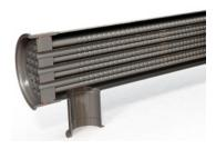
The HRS MR Series is a complete stainless steel shell and tube heat exchanger designed for hygienic applications. The product flows through both the inner tube and the surrounding shell for regeneration duties. The removable tubes allow hygienic processing on the shell side.
