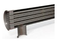
The HRS MR Series is a complete stainless steel shell and tube heat exchanger designed for hygienic applications. The product flows through both the inner tube and the surrounding shell for regeneration duties. The removable tubes allow hygienic processing on the shell side.
