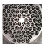
The HRS Unicus Series is a scraped surface heat exchanger was originally developed for food and hygienic applications. Based on the traditional shell and tube heat exchanger, the Unicus has scraping elements inside each interior tube which move back and forth by hydraulic action.
