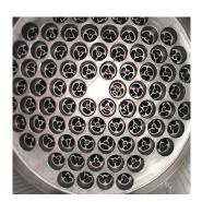
The HRS Unicus Series is a scraped surface heat exchanger was originally developed for food and hygienic applications. Based on the traditional shell and tube heat exchanger, the Unicus has scraping elements inside each interior tube which move back and forth by hydraulic action.
