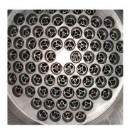
The HRS Unicus Series is a scraped surface heat exchanger was originally developed for food and sanitary applications. Based on the traditional shell and tube heat exchanger, the Unicus has scraping elements inside each interior tube which move back and forth by hydraulic action.
