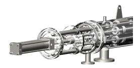
The HRS Unicus Series is a scraped surface heat exchanger ideal for food and hygienic applications. Based on the traditional shell and tube heat exchanger, the Unicus has scraping elements inside each interior tube which move back and forth by hydraulic action.
