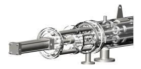
The HRS Unicus Series is a scraped surface heat exchanger ideal for food and sanitary applications. Based on the traditional shell and tube heat exchanger, the Unicus has scraping elements inside each interior tube which move back and forth by hydraulic action.
