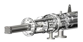
The HRS Unicus Series is a scraped surface heat exchanger ideal for food and hygienic applications. Based on the traditional shell and tube heat exchanger, the Unicus has scraping elements inside each interior tube which move back and forth by hydraulic action.
